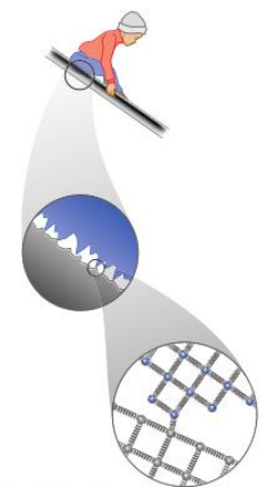
Figure 4.24 Friction is caused by bonds between atoms that form between the "high points" of the two surfaces that come into contact.
